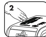
Touch test area and N look for the SafeSense® indicator to illuminate
